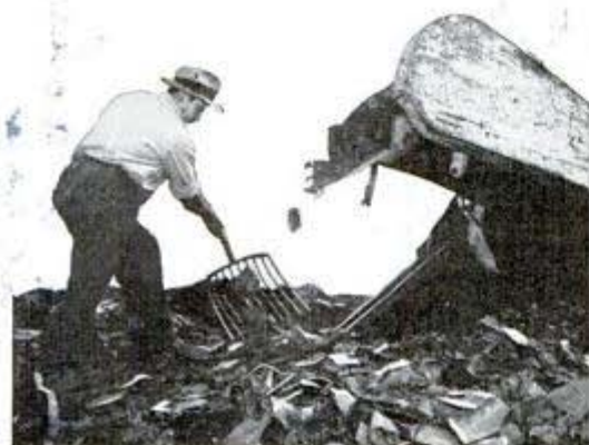
Sorting the scrap iron and steel with a fork as it drops from the endless conveyor
